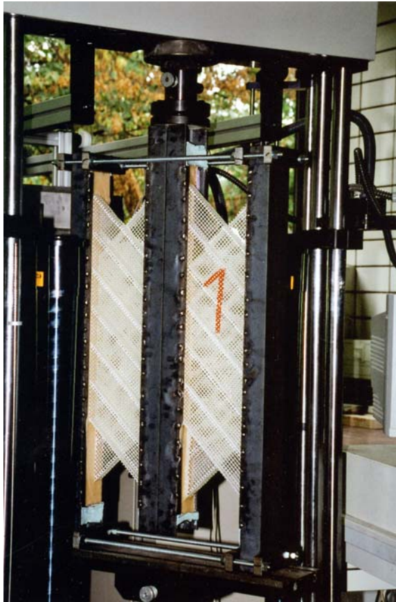
Fig. 3: Shear load test with a two layer \pm 45^\circ PEKATEX®-Strut configuration
